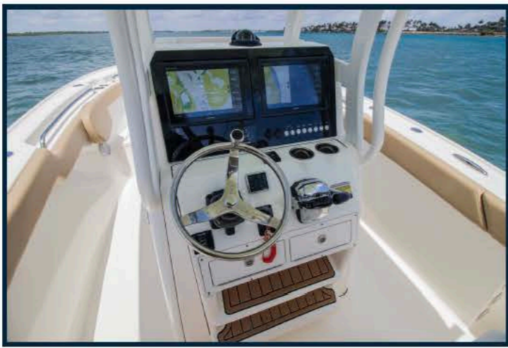
Large black dash to reduce glare and provide enough mounting surface for the new larger MFD's.
