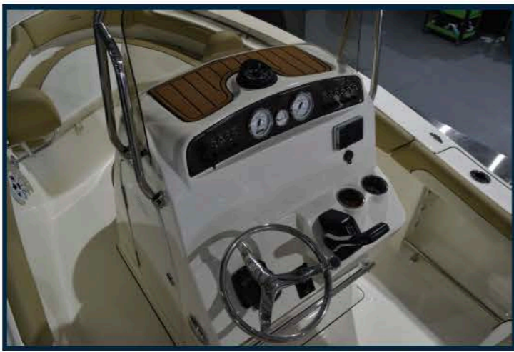
SeaDek padded console top with lighted compass, large flat mounting surface for today's larger MFD's, SeaStar tilt hydraulic steering and SS folding footrest are all standard features.
