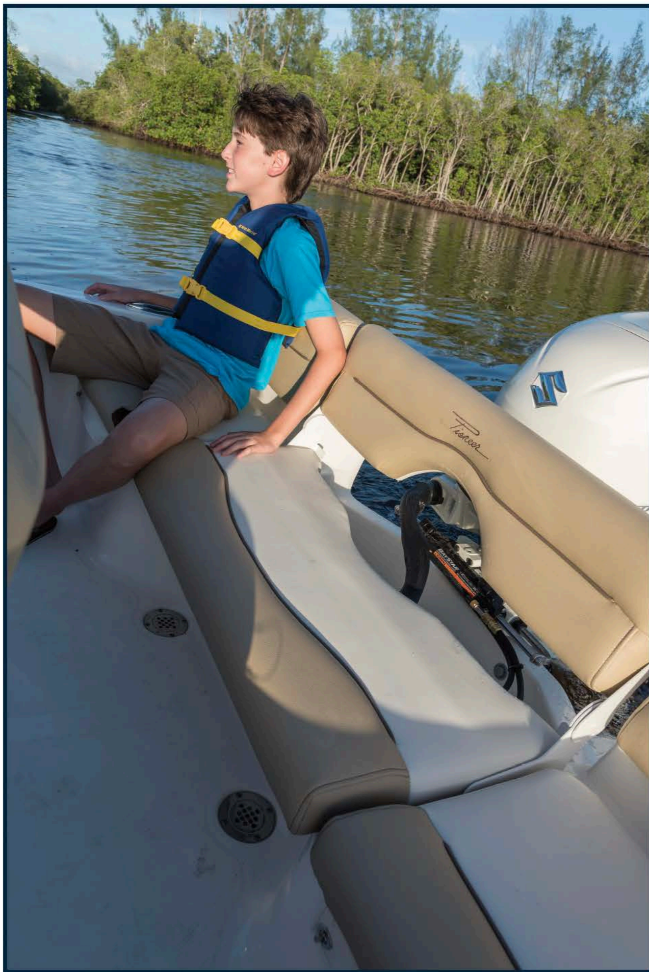
Full width stern bench seat that folds down for easy access to the swim platform.
