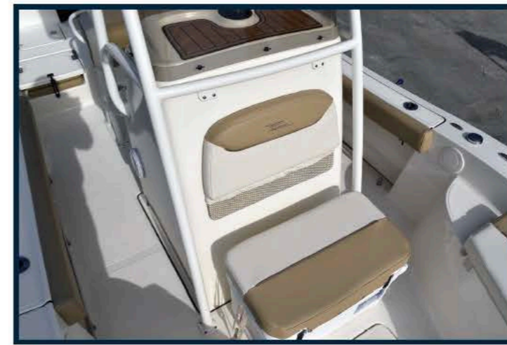
Console mounted t-top supports give the most floor space possible.
