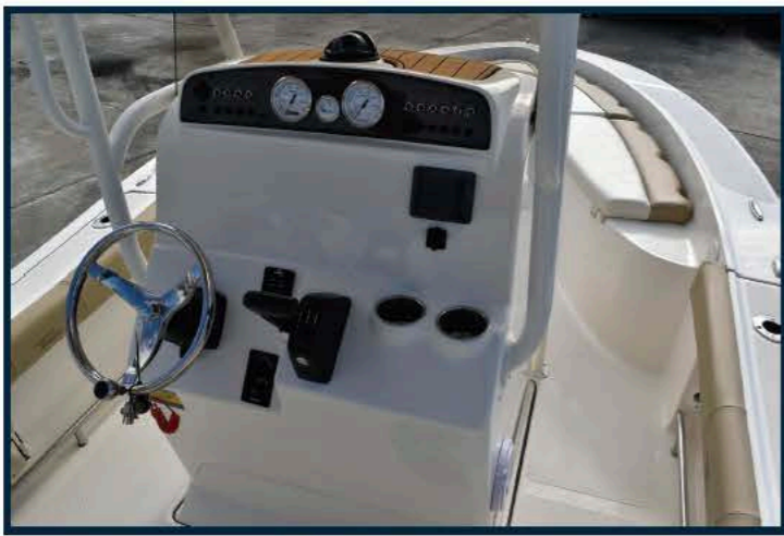
The console features a flat dash surface for today's larger electronics, 1" SS removable handrail, removable windshield, 12v power outlet, SS cupholders & SeaDek covering to protect your small items.
