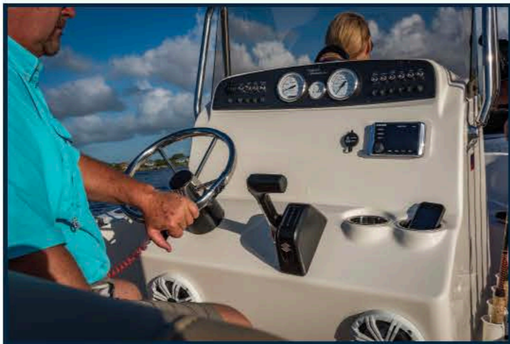
Flat dash surface for today's larger electronics, 1" SS removable handrail, removable windshield, 12v power outlet, SS cupholders and SeaDek covering to help protect small items.
