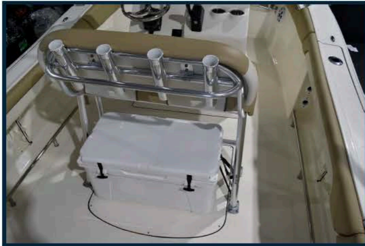
Standard rotomolded cooler under leaning post, SS toerails and bolsters wrapped all the way around the interior.
