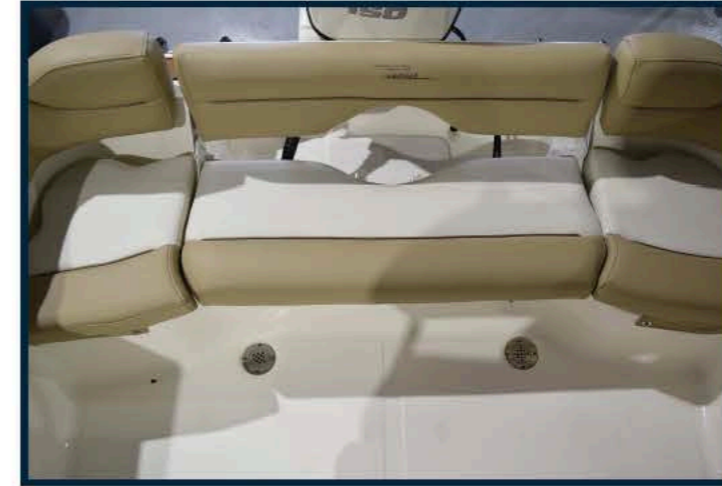
Full stern wrap around bench with folding backrest and SS scupper drains with check balls to provide a self baling cockpit.
