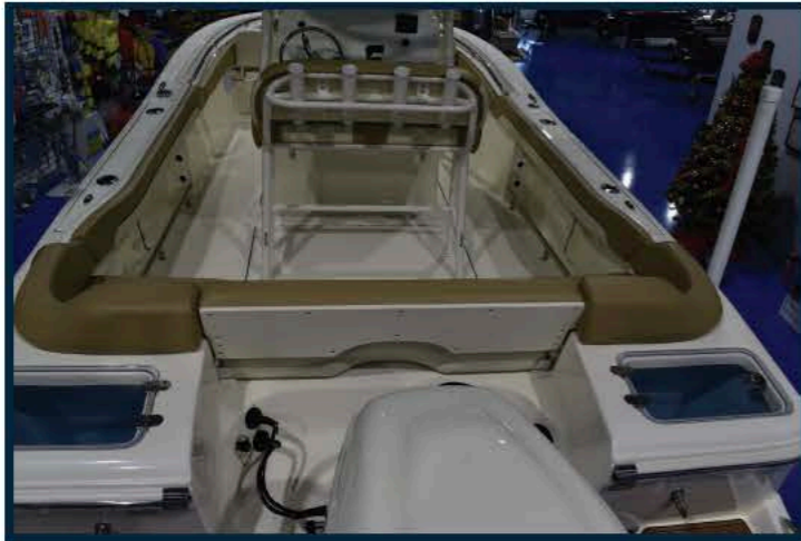
Port side 18 gallon livewell with blue interior standard, starboard side optional. SS toerail in the cockpit sole to provide security while docking, fighting or landing a fish.
