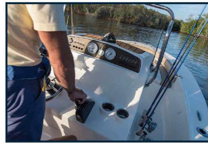
The console features a flat dash surface for today's larger electronics, 1" SS removable handrail, removable windshield, 12v power outlet, SS cupholders and SeaDek covering to help protect items like cell phone, handheld VHF radio 7 other small items that you want to keep handy at all times.
