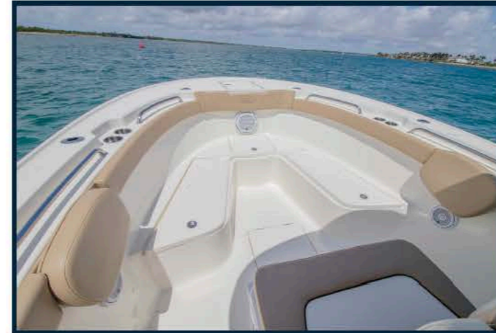
Horseshoe shaped bow seating with folding forward facing backrest and under seat storage that drains overboard. Recessed handrails and cup holders for safety and comfort. In floor storage for larger items.
