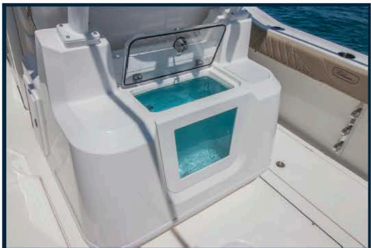
55 gallon aquarium style livewell in the leaning post to help keep weight forward and on the centerline of the boat to improve handling.
